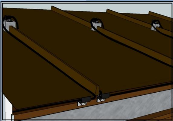
Using our Belt Clips to hold the wire below the roofing panel is a simple solution to avoiding loose fitting cables that can be a possible problem when ice slides down the metal roof cavity.
